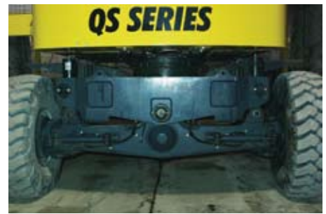
Parker's gas struts help keep the axles on the ground.
