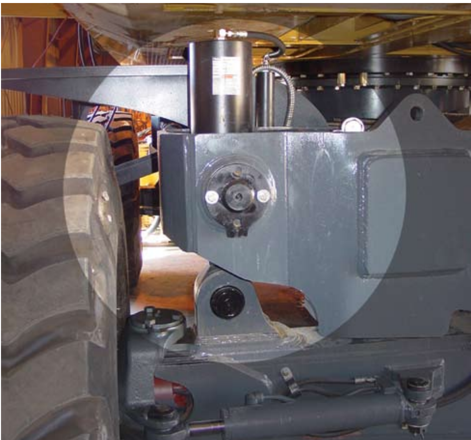
A close-up of Parker's Accumulator GaStrut on the BTI QS45 Series scaler, built for work in underground mines.
