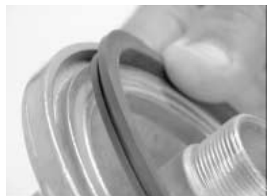
Installing the lip seal with the lip first into the LHA filter housing groove.
