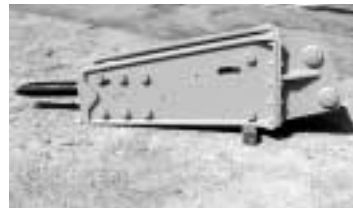
Breaker's mounting end elevated
