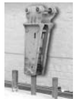
Breaker in Safety Stand
